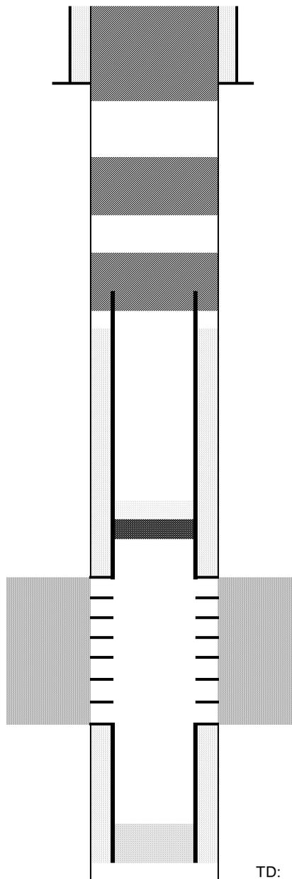
Cut surface casing off 6'-8' below surface.
