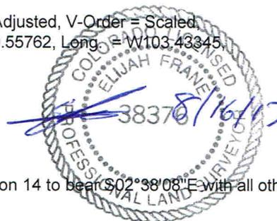
**Basis of Bearing:** Bearings were determined based on the West line of Section 14 to bear **S02°38'08"E** with all other bearings contained herein relative thereto.
