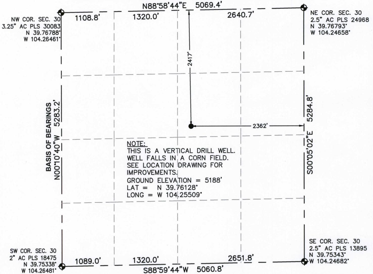
I HEREBY STATE TO SOUTHWESTERN ENERGY COMPANY THAT THE SURFACE LOCATION OF THE WELL LINNEBUR FLYING SERVICE 3-61 #1-30 IS LOCATED 2417 FEET FROM THE NORTH LINE AND 2362 FEET FROM THE EAST LINE, SECTION 30, T.3S., R.61W., 6TH P.M. FOR AND ON BEHALF OF NV5, INC.
