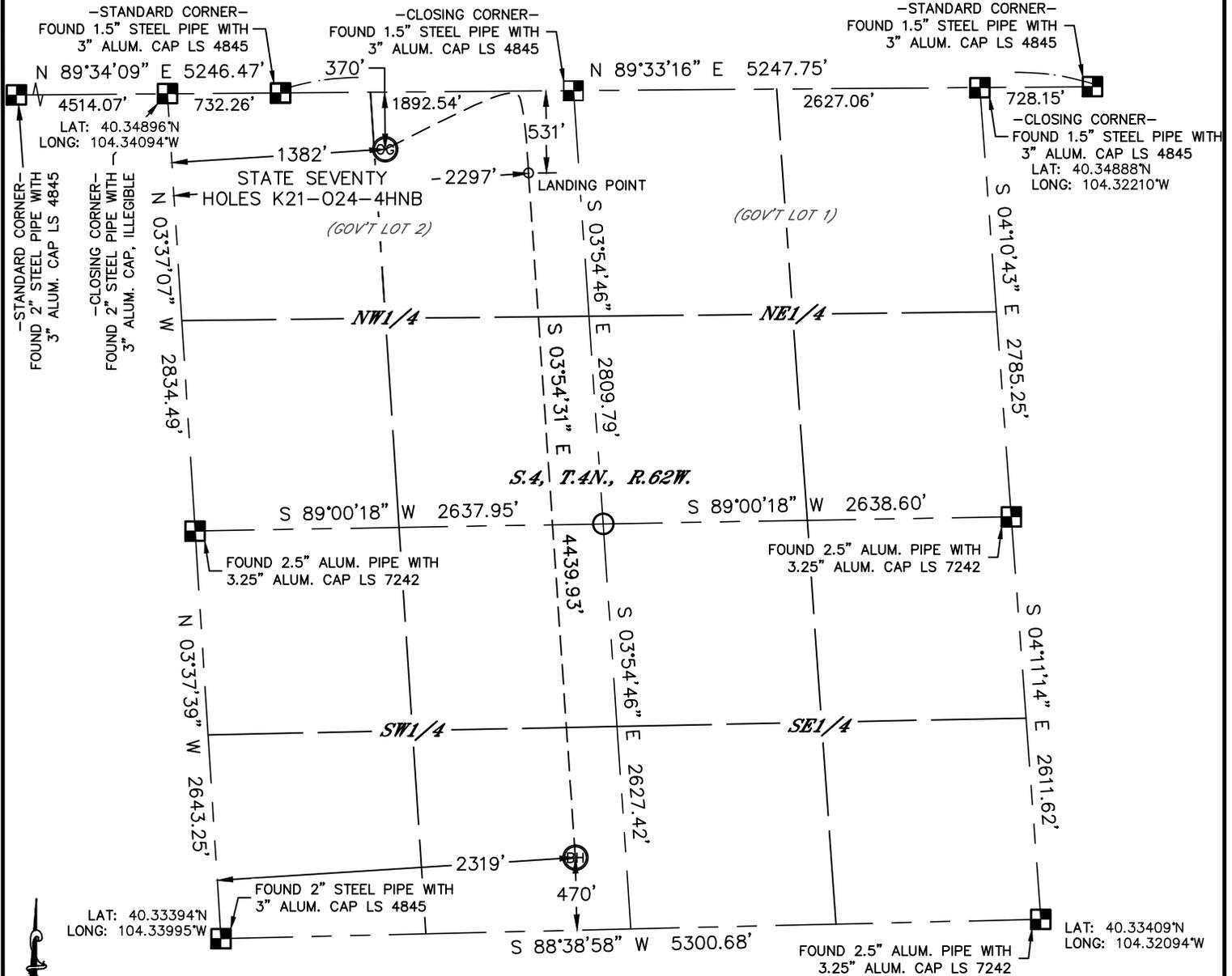
In accordance with a request from Keith Caplan with BONANZA CREEK ENERGY, INC. Lat40°, Inc. has determined the surface location of the STATE SEVENTY HOLES K21-024-4HNB to be 370' from the NORTH line and 1382' from the WEST line and the bottom hole to be 470' from the SOUTH line and 2319' from the WEST line as measured at right angles from the section lines of Section 4, Township 4 North, Range 62 West of the Sixth Principal Meridian, County of Weld, State of Colorado.
