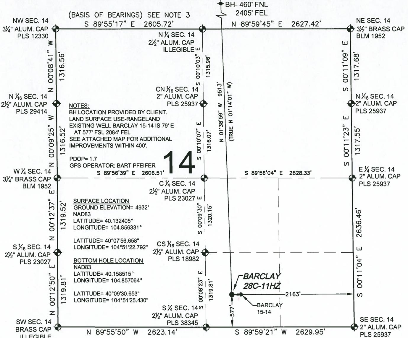
WELL BARCLAY 28C-11HZ TO BE LOCATED 577' FSL AND 2163' FEL
