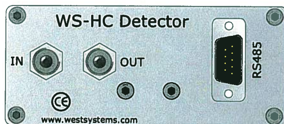
RS485 Connector DB9 Male panel
