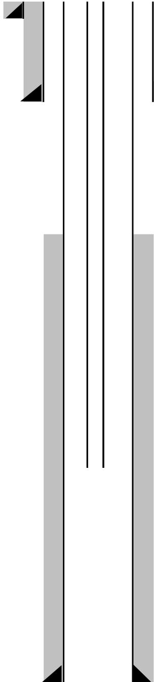
Conductor 26" Hole 18" casing/liner 42' W/ 16 Sks cmt
