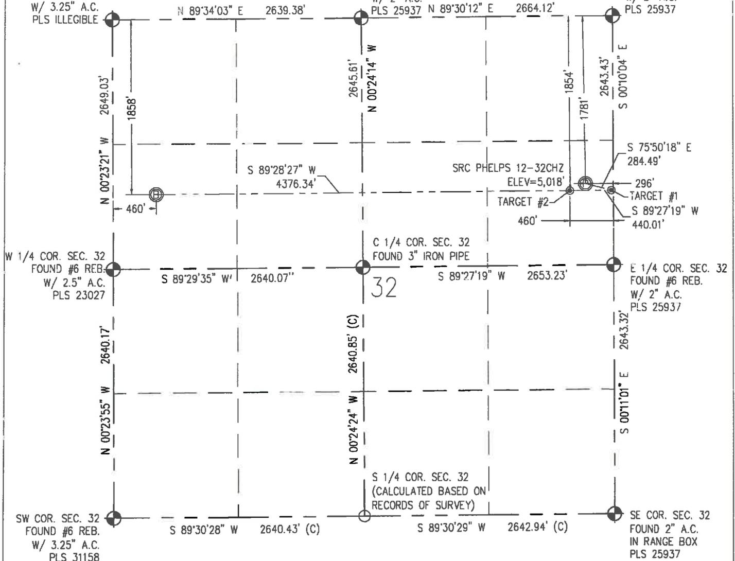
IN ACCORDANCE WITH A REQUEST FROM CRAIG RASMUSON - SYNERGY RESOURCES, BASELINE ENGINEERING CORP. HAS DETERMINED THE LOCATION OF THE SRC PHELPS 12-32CHZ TO BE 1,781' FNL AND 296' FEL, AS MEASURED AT NINETY (90) DEGREES FROM THE SECTION LINE OF SECTION 32, TOWNSHIP 1 NORTH, RANGE 66 WEST AND THE BOTTOM HOLE LOCATION TO BE 1,858' FNL AND 460' FNL OF SECTION 32, TOWNSHIP 1 NORTH, RANGE 66 WEST, 6TH PRINCIPAL MERIDIAN, WELD COUNTY, COLORADO.
