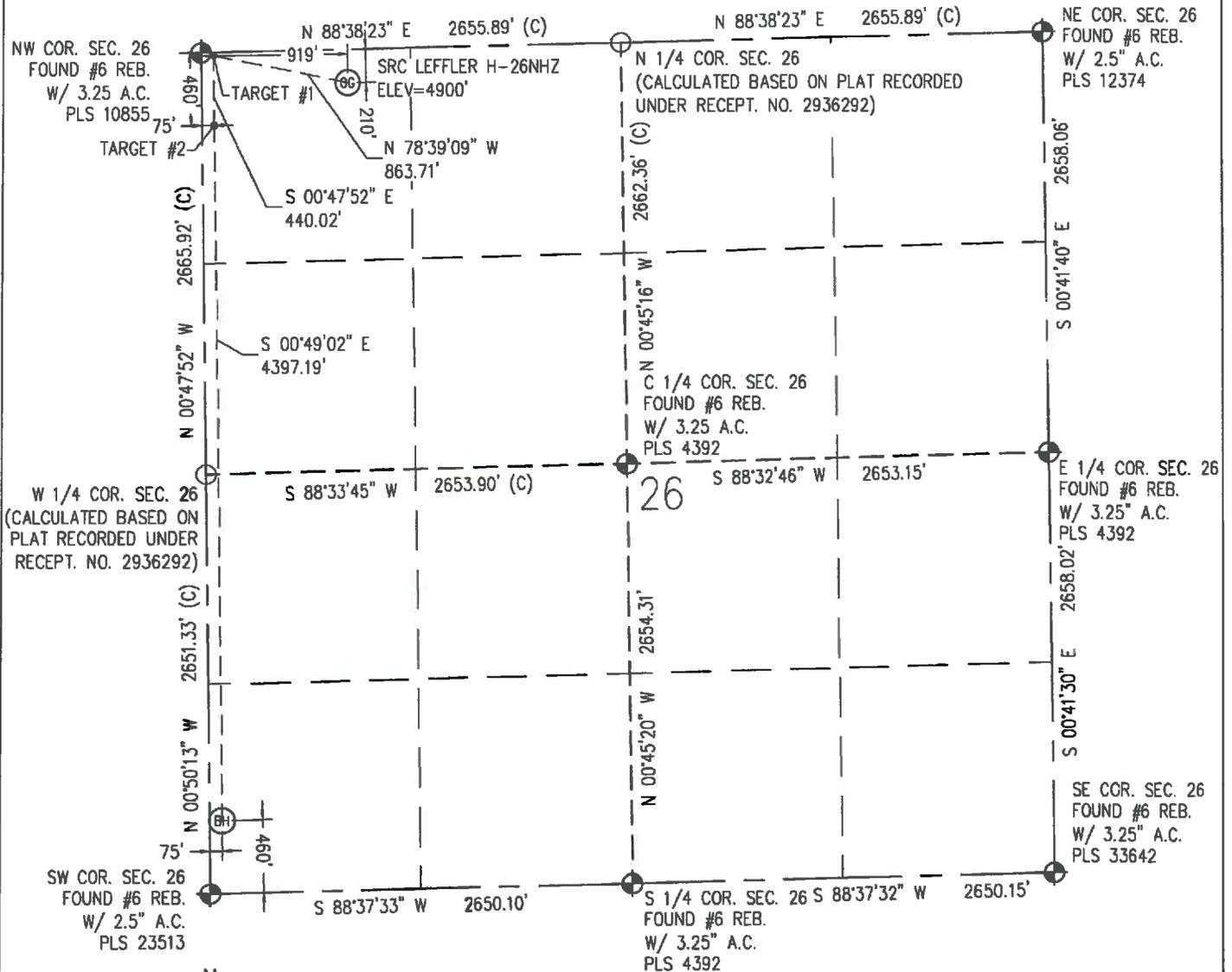
IN ACCORDANCE WITH A REQUEST FROM CRAIG RASMUSON - SYNERGY RESOURCES, BASELINE ENGINEERING CORP. HAS DETERMINED THE LOCATION OF THE SRC LEFFLER H-26NHZ TO BE 210' FNL AND 919' FWL, AS MEASURED AT NINETY (90) DEGREES FROM THE SECTION LINE OF SECTION 26, TOWNSHIP 7 NORTH, RANGE 66 WEST AND THE BOTTOM HOLE LOCATION TO BE 460' FSL AND 75' FWL OF SECTION 26, TOWNSHIP 7 NORTH, RANGE 66 WEST, 6TH PRINCIPAL MERIDIAN, WELD COUNTY, COLORADO
