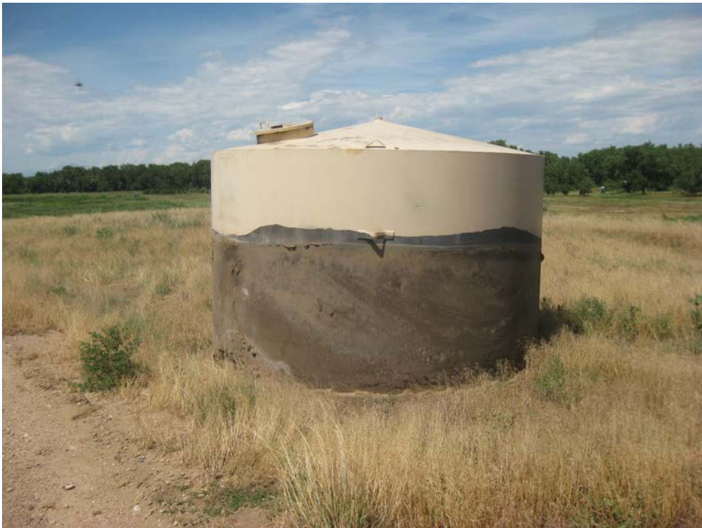
Steel water pit after removal. No indication of failure was observed.
