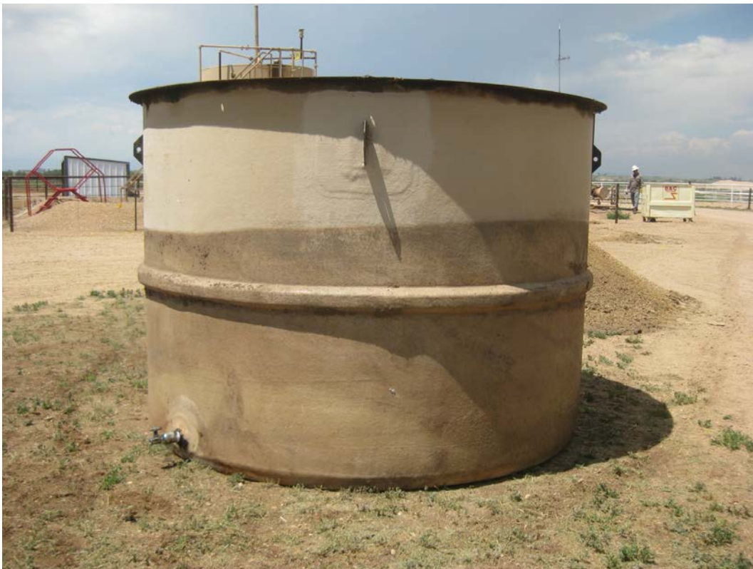
Fiberglass water pit after removal. No obvious indication of failure was noted.
