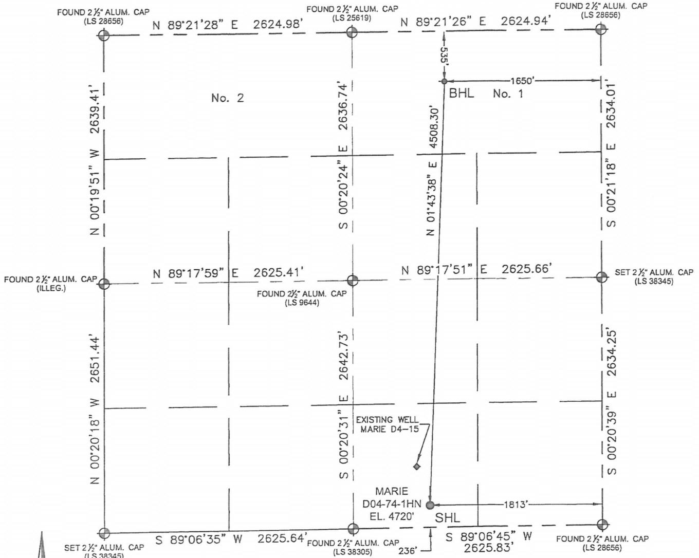
In accordance with a request from Derrick Worden with Noble Energy Inc. Petroleum Field Services, LLC has determined the surface location of the **MARIE D04-74-1HN** to be 236' from the SOUTH line and 1813' from the EAST line and the bottom hole to be 535' from the NORTH line and 1650' from the EAST line as measured at right angles from the section line of Section 4, Township 3 North, Range 64 West of the Sixth Principal Meridian, County of WELD, State of Colorado.
