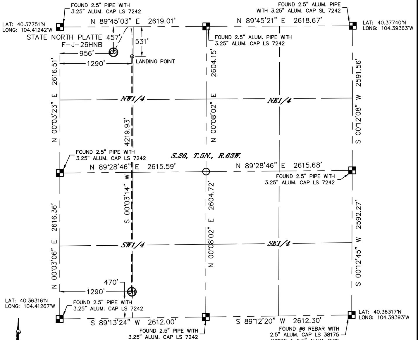
In accordance with a request from Michael Meagher with BONANZA CREEK ENERGY, INC. Lat40°, Inc. has determined the surface location of the STATE NORTH PLATTE F-J-26HNB to be 457' from the NORTH line and 956' from the WEST line and the bottom hole to be 470' from the SOUTH line and 1290' from the WEST line as measured at right angles from the section lines of Section 26, Township 5 North, Range 63 West of the Sixth Principal Meridian, County of Weld, State of Colorado.
