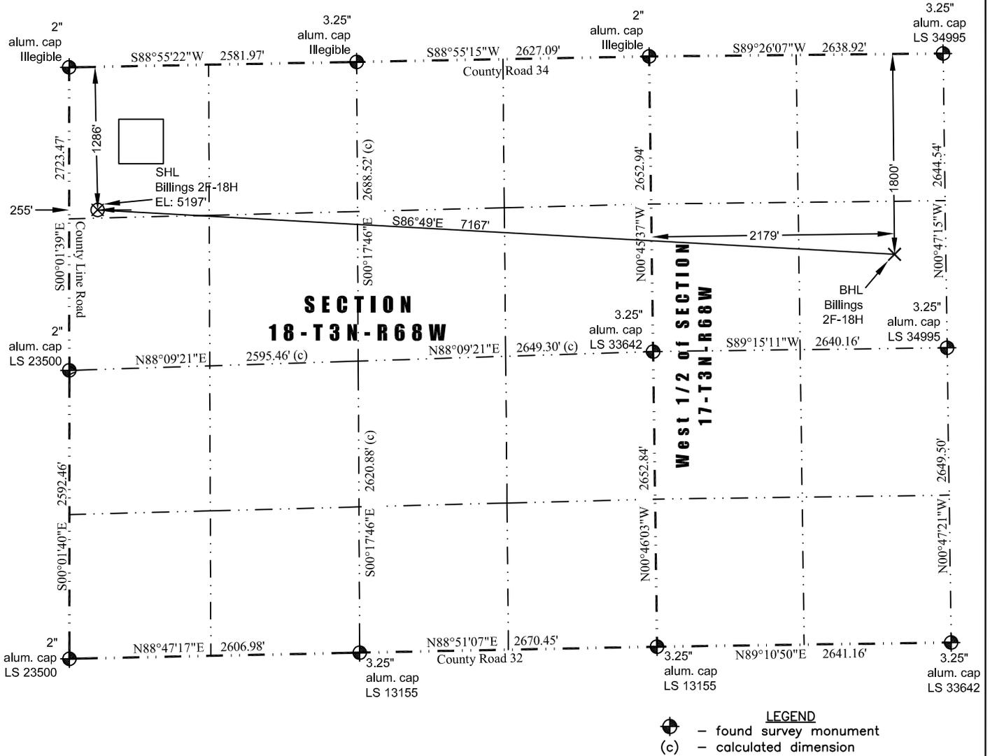
In accordance with a request from Jay Knutson of EnCana Oil & Gas (USA) Inc., JR Land Surveying, LLC has determined the location of the **Billings 2F-18H** well site to be SHL: 1286' FNL and 255' FWL, (BHL: 1800' FNL and 2179' FWL) as measured at ninety (90) degrees from the section lines of Section 18 and Section 17, Township 3 North, Range 68 West, 6th Principal Meridian, County of Weld, CO.
