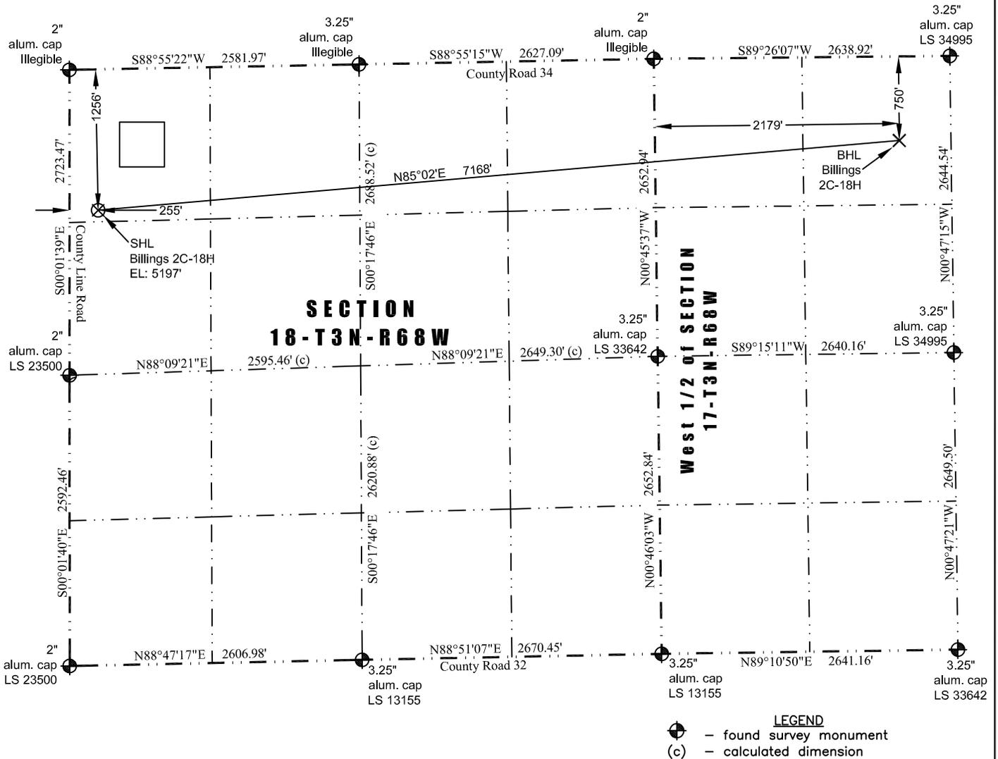
In accordance with a request from Jay Knutson of EnCana Oil & Gas (USA) Inc., JR Land Surveying, LLC has determined the location of the **Billings 2C-18H** well site to be SHL: 1256' FNL and 255' FWL, (BHL: 750' FNL and 2179' FWL) as measured at ninety (90) degrees from the section lines of Section 18 and Section 17, Township 3 North, Range 68 West, 6th Principal Meridian, County of Weld, CO.
