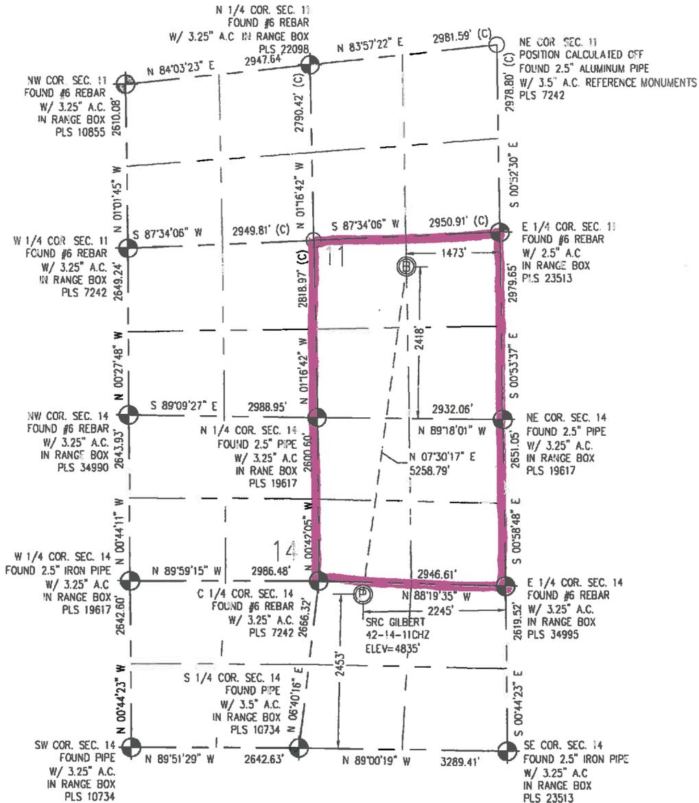
IN ACCORDANCE WITH A REQUEST FROM CRAIG RASMUSON - SYNERGY RESOURCES, BASELINE ENGINEERING CORP. HAS DETERMINED THE LOCATION OF THE SRC GILBERT 42-14-11CHZ TO BE 2,453' FSL AND 2,245' FEL, AS MEASURED AT NINETY (90) DEGREES FROM THE SECTION LINE OF SECTION 14, TOWNSHIP 5 NORTH, RANGE 66 WEST AND THE BOTTOM HOLE LOCATION TO BE 2,418' FSL AND 1,473' FEL OF SECTION 11, TOWNSHIP 5 NORTH, RANGE 66 WEST, 6TH PRINCIPAL MERIDIAN, WELD COUNTY, COLORADO.
