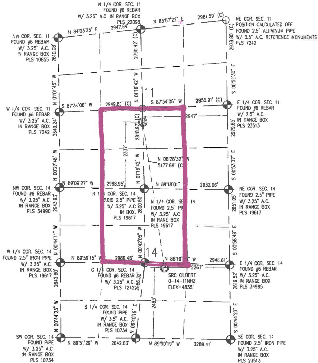
IN ACCORDANCE WITH A REQUEST FROM CRAIG RASMUSON - SYNERGY RESOURCES, BASELINE ENGINEERING CORP. HAS DETERMINED THE LOCATION OF THE SRC GILBERT 0-14-11NHZ TO BE 2,483' FSL AND 2,267' FEL, AS MEASURED AT NINETY (90) DEGREES FROM THE SECTION LINE OF SECTION 14, TOWNSHIP 5 NORTH, RANGE 66 WEST AND THE BOTTOM HOLE LOCATION TO BE 2,337' FSL AND 2,947' FEL OF SECTION 11, TOWNSHIP 5 NORTH, RANGE 66 WEST, 6TH PRINCIPAL MERIDIAN, WELD COUNTY, COLORADO
