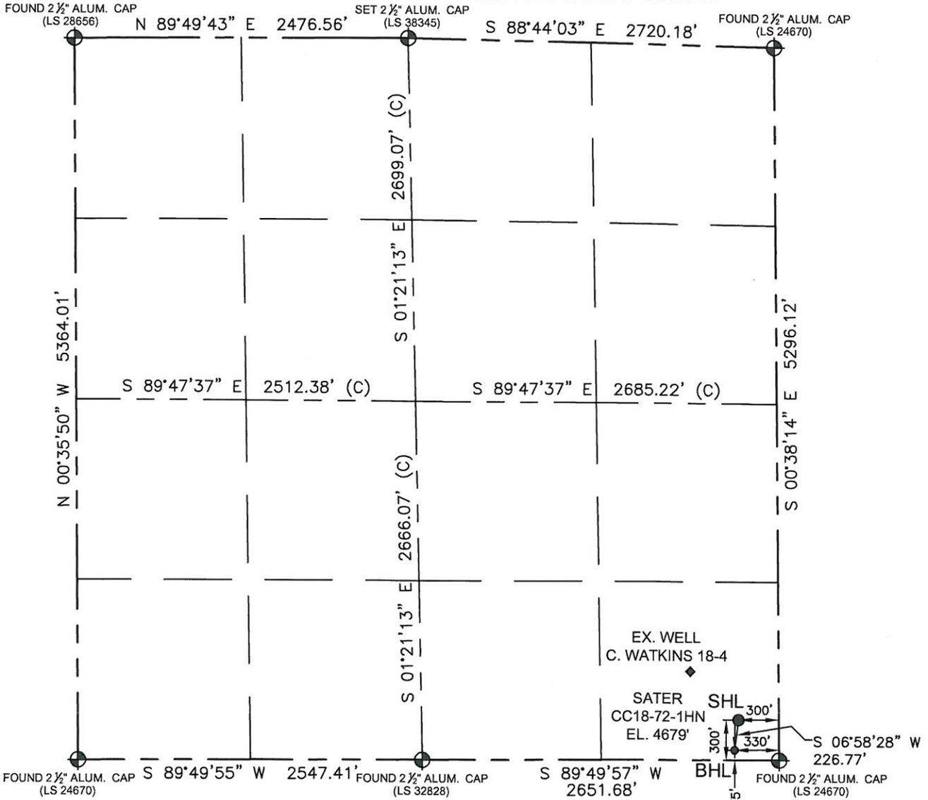
In accordance with a request from Matt Verbit with Noble Energy Inc. Petroleum Field Services, LLC has determined the surface location of the SATER CC18-72-1HN to be 300' from the SOUTH line and 300' from the EAST line and the bottom hole to be 75' from the SOUTH line and 330' from the EAST line as measured at right angles from the section line of Section 18, Township 4 North, Range 63 West of the Sixth Principal Meridian, County of WELD, State of Colorado.
