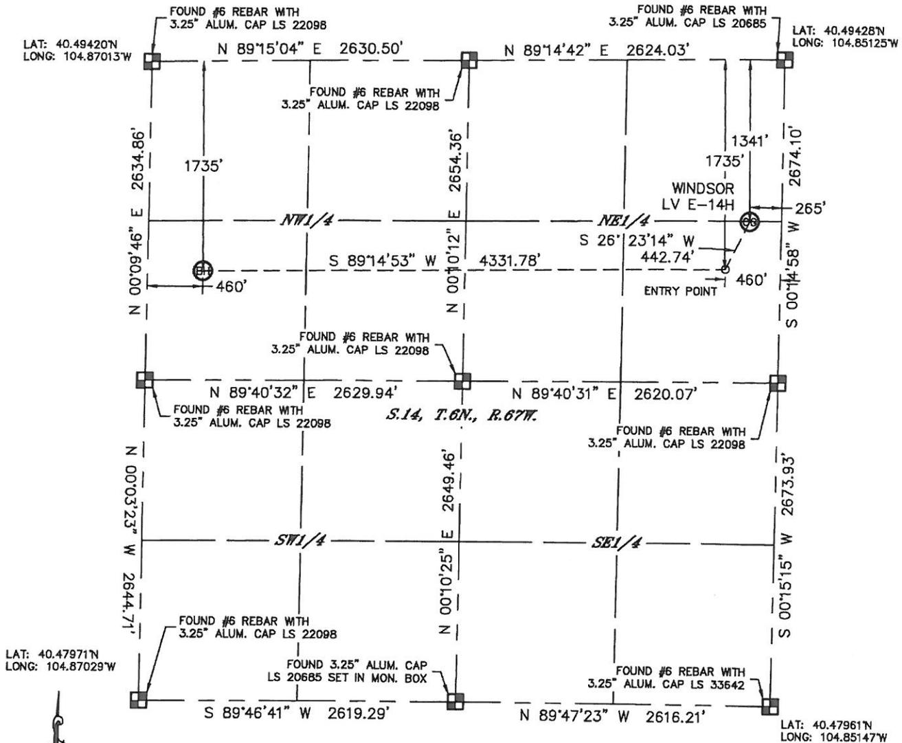
In accordance with a request from Jesse White with APOLLO OPERATING, LLC, Lat40°, Inc. has determined the surface location of the WINDSOR LV E-14H to be 1341' from the NORTH line and 265' from the EAST line and the bottom hole to be 1735' from the NORTH line and 460' from the WEST line as measured at right angles from the section lines of Section 14, Township 6 North, Range 67 West of the Sixth Principal Meridian, County of Weld, State of Colorado.
