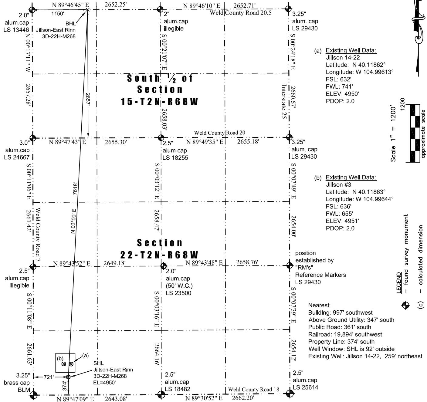
In accordance with a request from Jay Knutson of EnCana Oil & Gas (USA) Inc., JR Land Surveying, LLC has determined the location of the **Jillson-East Rinn 3D-22H-M268** well site to be SHL: 374' FSL and 721' FWL, (BHL: 2657' FSL and 1150' FWL), as measured at ninety (90) degrees from the section lines of Sections 15 and 22, Township 2 North, Range 68 West of the 6th Principal Meridian, Weld County Colorado.
