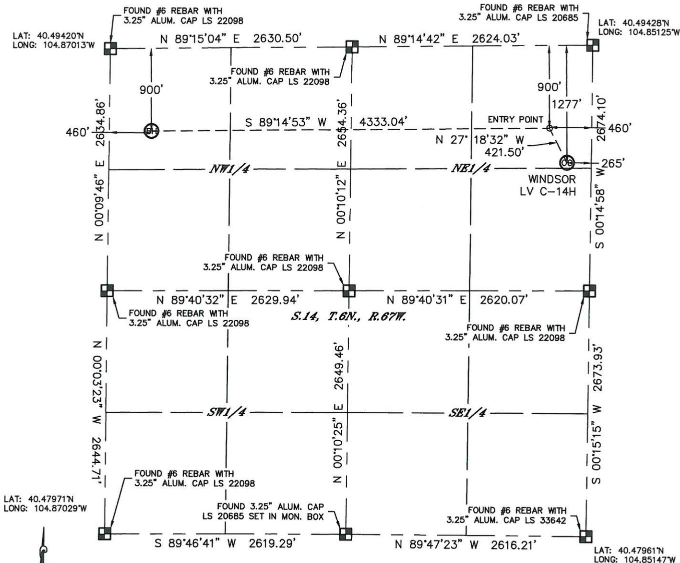
In accordance with a request from Jesse White with APOLLO OPERATING, LLC. Lat40°, Inc. has determined the surface location of the WINDSOR LV C-14H to be 1277' from the NORTH line and 265' from the EAST line and the bottom hole to be 900' from the NORTH line and 460' from the WEST line as measured at right angles from the section lines of Section 14, Township 6 North, Range 67 West of the Sixth Principal Meridian, County of Weld, State of Colorado.
