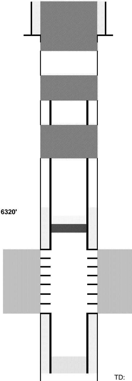
Cut surface casing off 6'-8' below surface.
