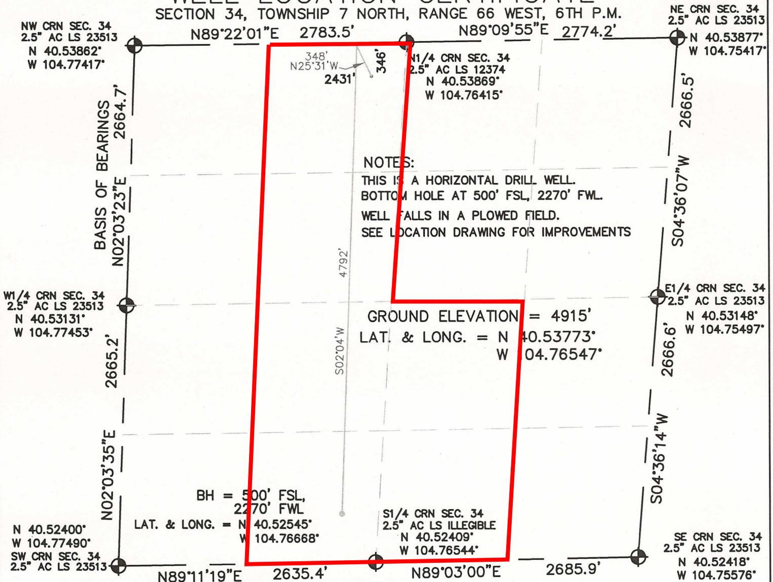
I HEREBY STATE TO PDC ENERGY THAT THE SURFACE LOCATION OF THE WELL ANDERSON 34M-343 IS LOCATED 346' FNL & 2431' FWL, SEC. 34, T7N, R66W, 6PM.
