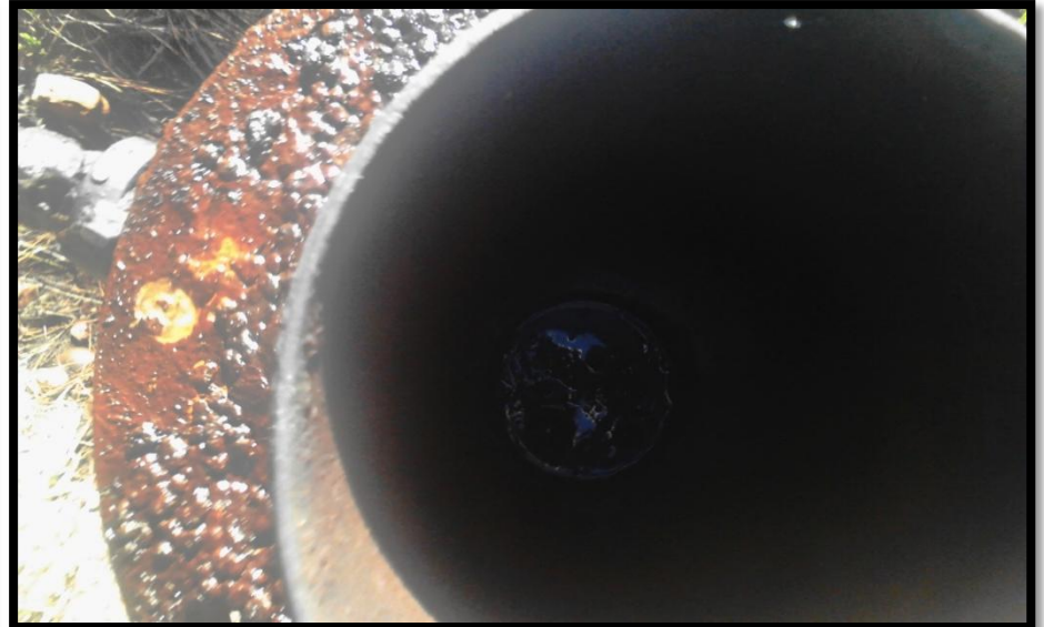
Interior view of production casing (~4'') showing present hydrostatic level of viscid brown oil. (bubbling at time of inspection).
