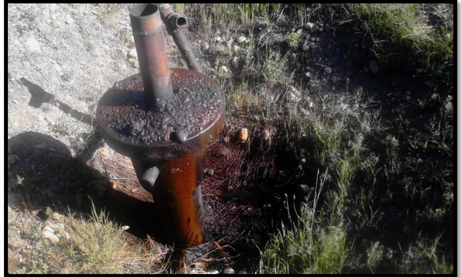
Close up view of oil saturation surrounding well piping exterior, casing-head, and adjacent soils and vegetation.
