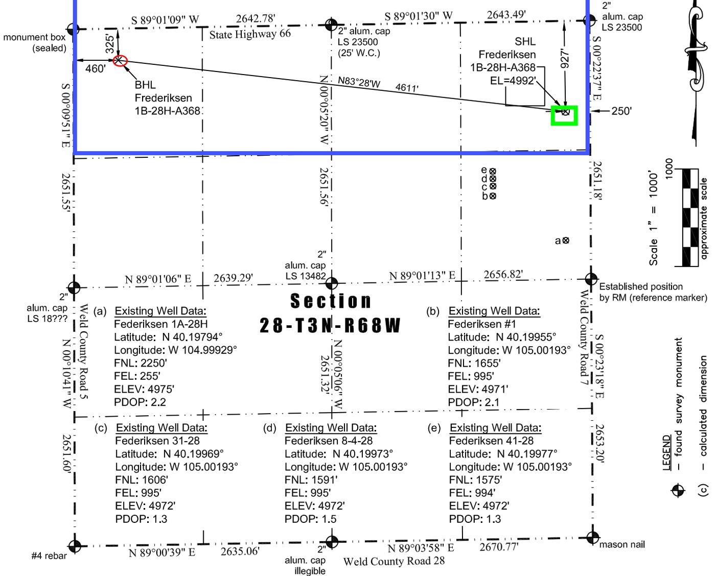
In accordance with a request from Jay Knutson of EnCana Oil & Gas (USA) Inc., JR Land Surveying, LLC has determined the location of the **Frederiksen 1B-28H-A368** well site to be SHL: 927' FNL and 250' FEL, (BHL: 325' FNL and 460' FWL), as measured at ninety (90) degrees from the section lines of Section 28, Township 3 North, Range 68 West of the 6th Principal Meridian, Weld County Colorado.
