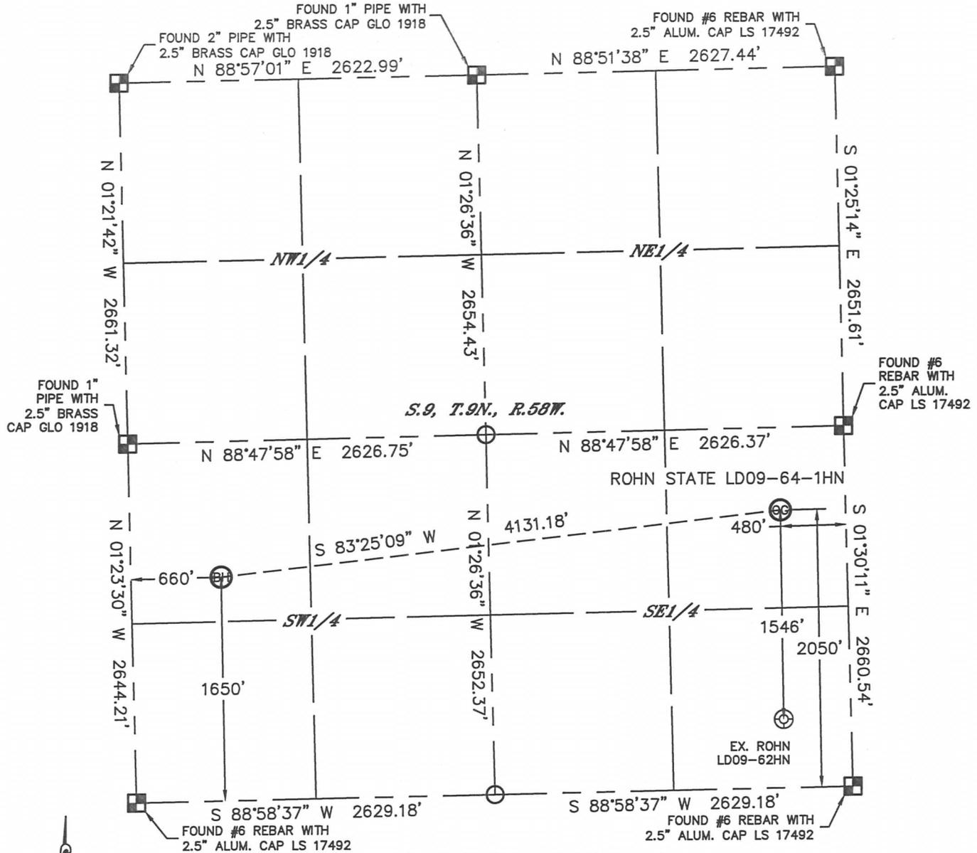
In accordance with a request from Derrick Worden with Noble Energy Inc. Lat40°, Inc. has determined the surface location of the ROHN STATE LD09-64-1HN to be 2050' from the SOUTH line and 480' from the EAST line and the bottom hole to be 1650' from the SOUTH line and 660' from the WEST line as measured at right angles from the section lines of Section 9, Township 9 North, Range 58 West of the Sixth Principal Meridian, County of Weld, State of Colorado.
