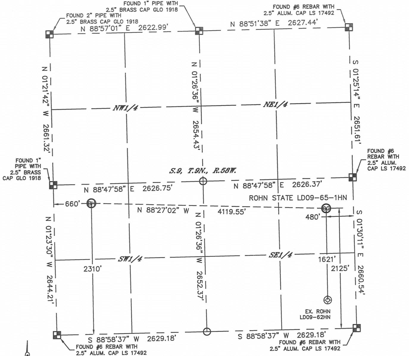
In accordance with a request from Derrick Worden with Noble Energy Inc. Lat40°, Inc. has determined the surface location of the ROHN STATE LD09-65-1HN to be 2125' from the SOUTH line and 480' from the EAST line and the bottom hole to be 2310' from the SOUTH line and 660' from the WEST line as measured at right angles from the section lines of Section 9, Township 9 North, Range 58 West of the Sixth Principal Meridian, County of Weld, State of Colorado.
