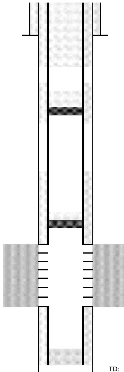
Cut surface casing off 6'-8' below surface.
