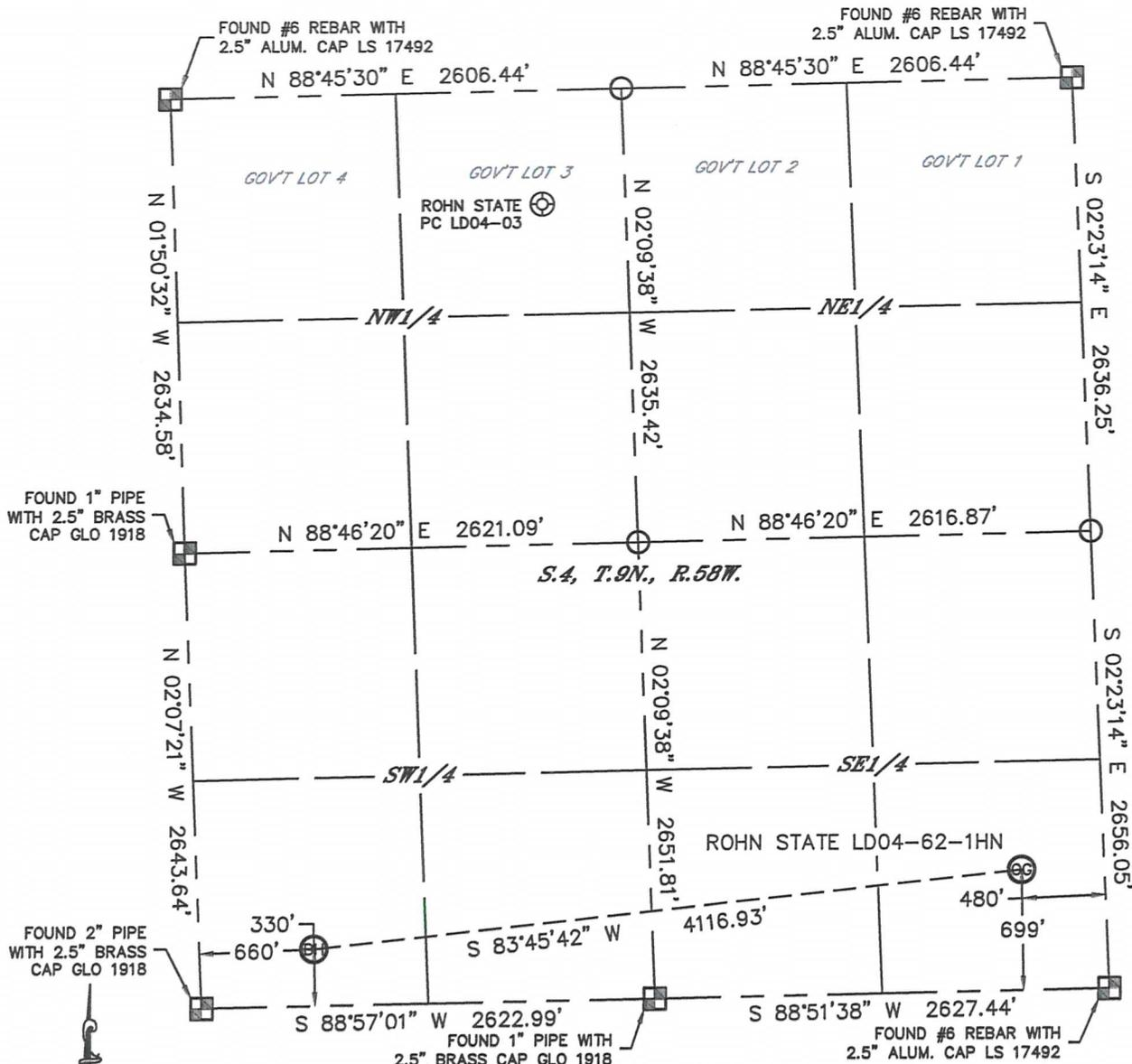
In accordance with a request from Nate McCorkell with Noble Energy Inc., Lat40°, Inc. has determined the surface location of the ROHN STATE LD04-62-1HN to be 699' from the SOUTH line and 480' from the EAST line and the bottom hole to be 330' from the SOUTH line and 660' from the WEST line as measured at right angles from the section lines of Section 4, Township 9 North, Range 58 West of the Sixth Principal Meridian, County of Weld, State of Colorado.
