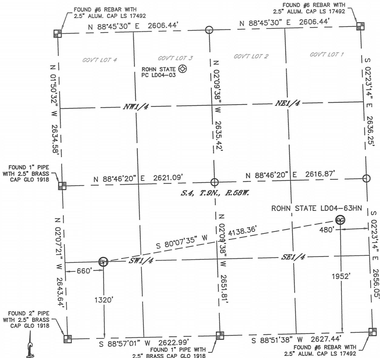
In accordance with a request from Nate McCorkell with Noble Energy Inc., Lat40°, Inc. has determined the surface location of the ROHN STATE LD04-63HN to be 1952' from the SOUTH line and 480' from the EAST line and the bottom hole to be 1320' from the SOUTH line and 660' from the WEST line as measured at right angles from the section lines of Section 4, Township 9 North, Range 58 West of the Sixth Principal Meridian, County of Weld, State of Colorado.
