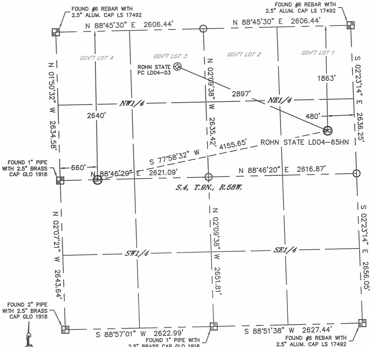
In accordance with a request from Nate McCorkell with Noble Energy Inc. Lat40°, Inc. has determined the surface location of the ROHN STATE LD04-65HN to be 1863' from the NORTH line and 480' from the EAST line and the bottom hole to be 2640' from the NORTH line and 660' from the WEST line as measured at right angles from the section lines of Section 4, Township 9 North, Range 58 West of the Sixth Principal Meridian, County of Weld, State of Colorado.
