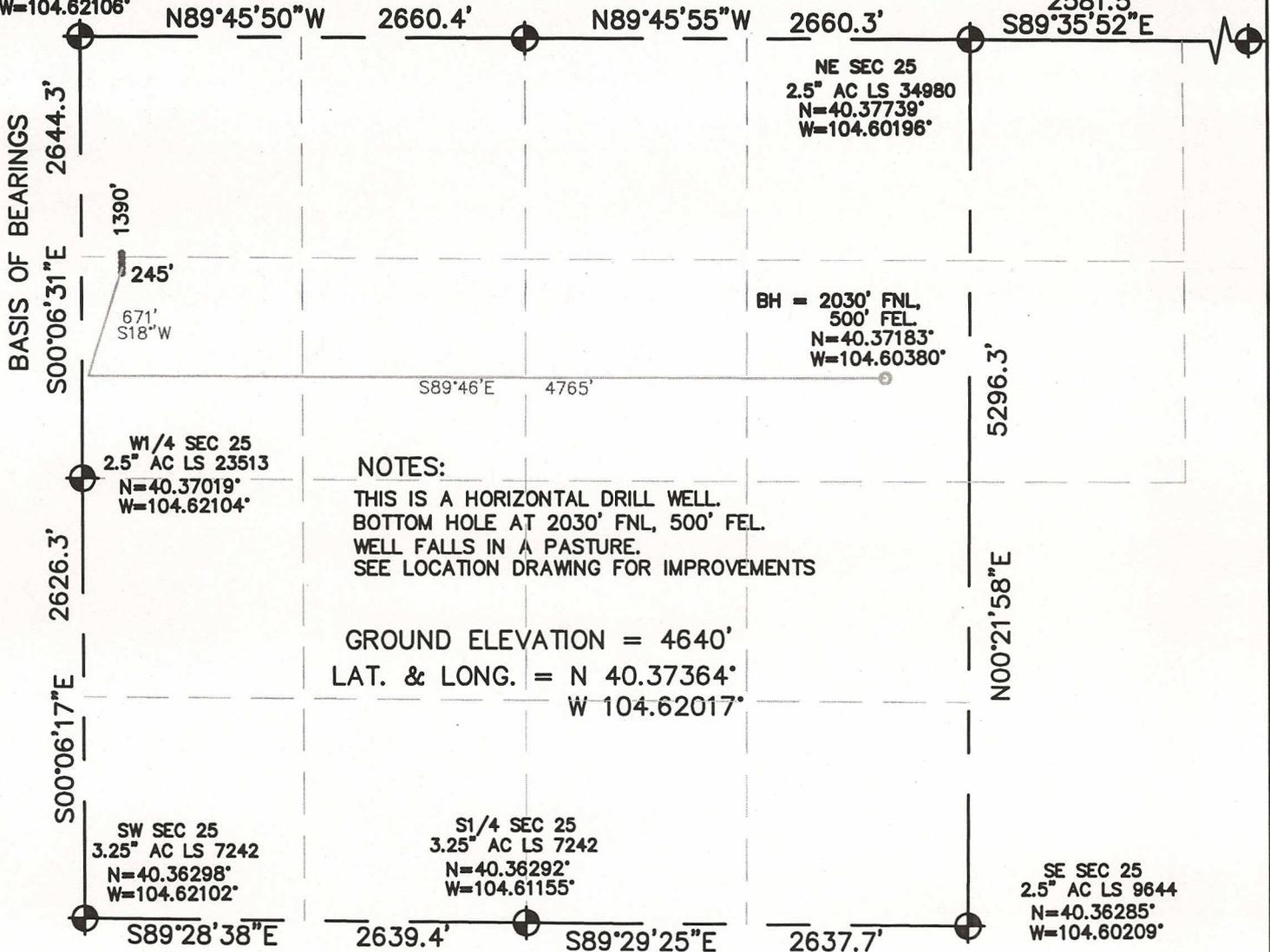
I HEREBY STATE TO PDC ENERGY THAT THE SURFACE LOCATION FOR THE WELL LASALLE 25G-212 IS LOCATED 1390' FNL & 245' FWL, SEC. 25, T5N, R65W, 6PM.
