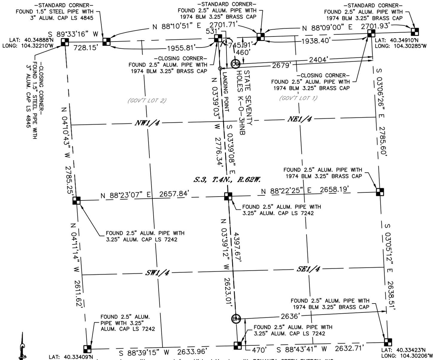
In accordance with a request from Michael Meagher with BONANZA CREEK ENERGY, INC. Lat40°, Inc. has determined the surface location of the STATE SEVENTY HOLES K-O-3HNB to be 460' from the NORTH line and 2404' from the EAST line and the bottom hole to be 470' from the SOUTH line and 2636' from the EAST line as measured at right angles from the section lines of Section 3, Township 4 North, Range 62 West of the Sixth Principal Meridian, County of Weld, State of Colorado.
