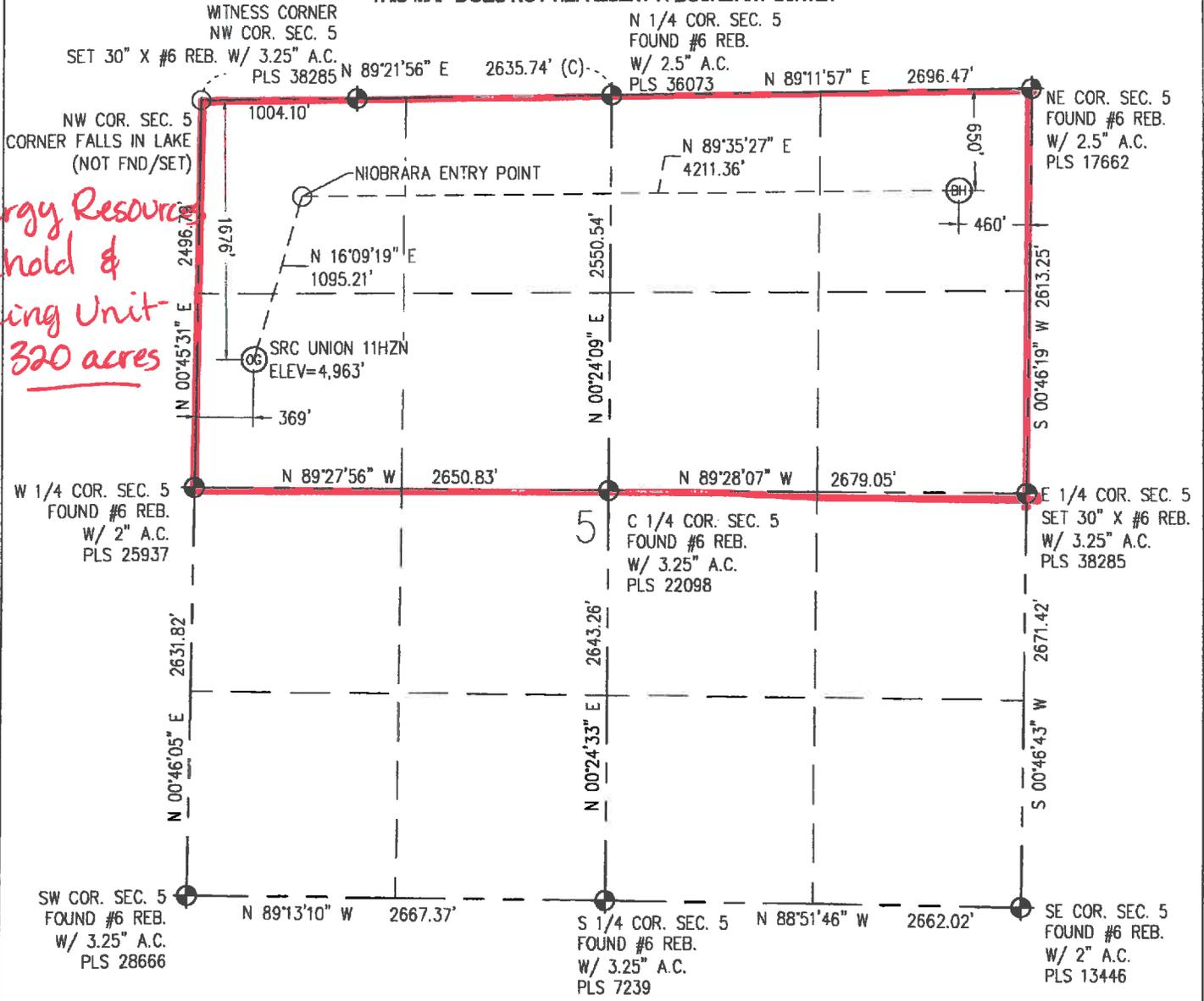
IN ACCORDANCE WITH A REQUEST FROM CRAIG RASMUSON - SYNERGY RESOURCES, BASELINE ENGINEERING CORP. HAS DETERMINED THE LOCATION OF THE SRC UNION 11HZN TO BE 1676' FNL AND 369' FWL, AS MEASURED AT NINETY (90) DEGREES FROM THE SECTION LINE OF SECTION 5, TOWNSHIP 2 NORTH, RANGE 68 WEST AND THE BOTTOM HOLE LOCATION TO BE 650' FNL AND 460' FWL OF SECTION 5, TOWNSHIP 2 NORTH, RANGE 68 WEST, 6TH PRINCIPAL MERIDIAN, WELD COUNTY, COLORADO.
