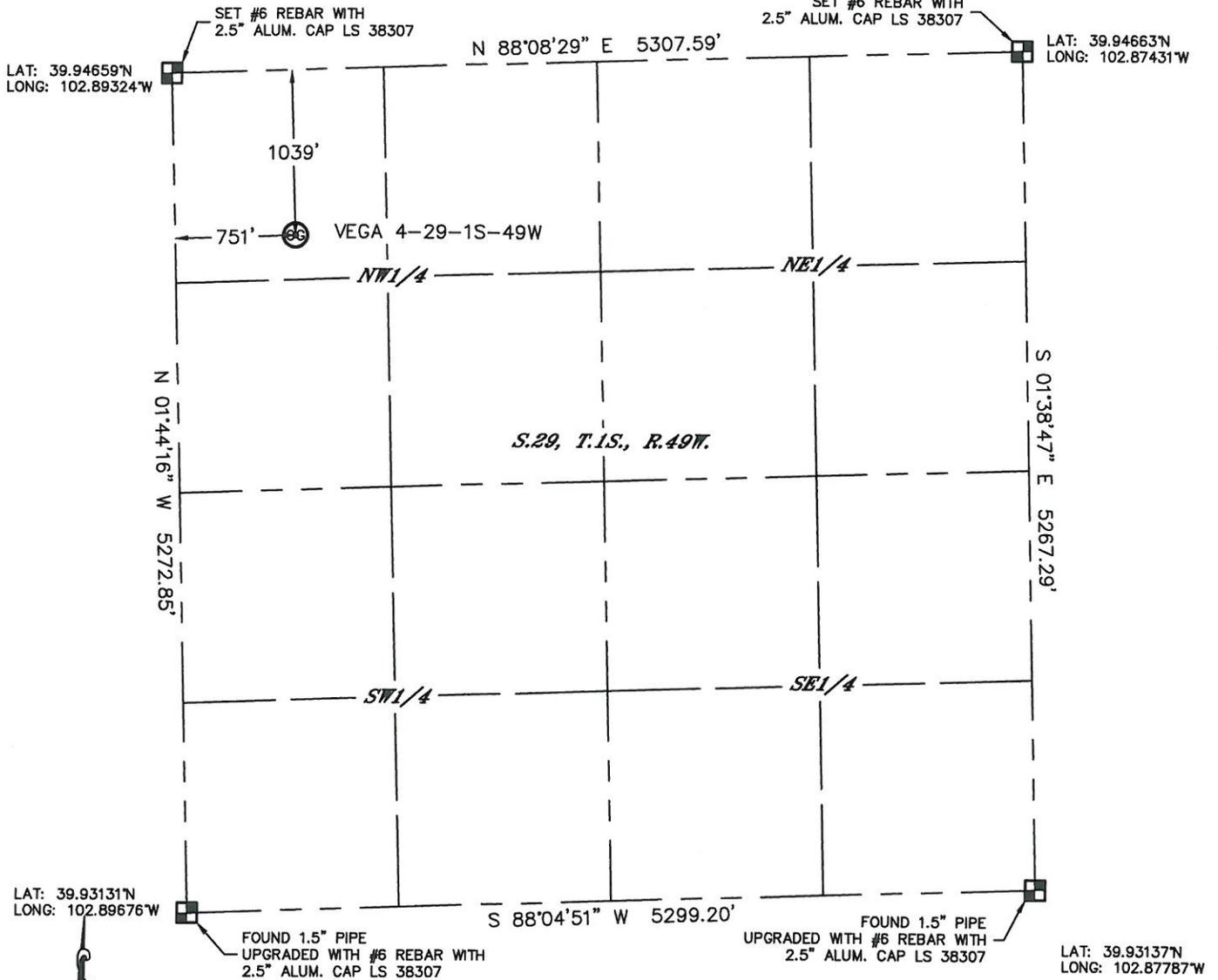
In accordance with a request from CLIFF WILLIAMS with OMIMEX PETROLEUM, INC. Lat40°, Inc. has determined the surface location of the VEGA 4-29-1S-49W to be 1039' from the NORTH line and 751' from the WEST line as measured at right angles from the section lines of Section 29, Township 1 South, Range 49 West of the Sixth Principal Meridian, County of Washington, State of Colorado.
