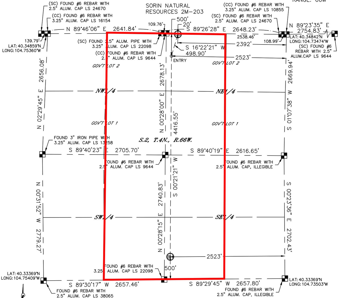
In accordance with a request from Jeff Dillingham with PDC ENERGY Lat40°, Inc. has determined the surface location of the SORIN NATURAL RESOURCES 2M-203 to be 20' from the NORTH line and 2392' from the EAST line and the bottom hole to be 500' from the SOUTH line and 2523' from the EAST line as measured at right angles from the section lines of Section 2, Township 4 North, Range 66 West of the Sixth Principal Meridian, County of Weld, State of Colorado.
