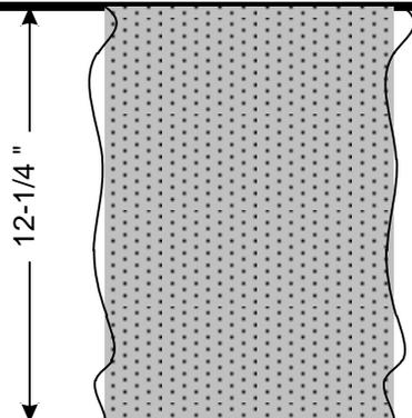
**12-1/4" Hole drilled to 312'**
