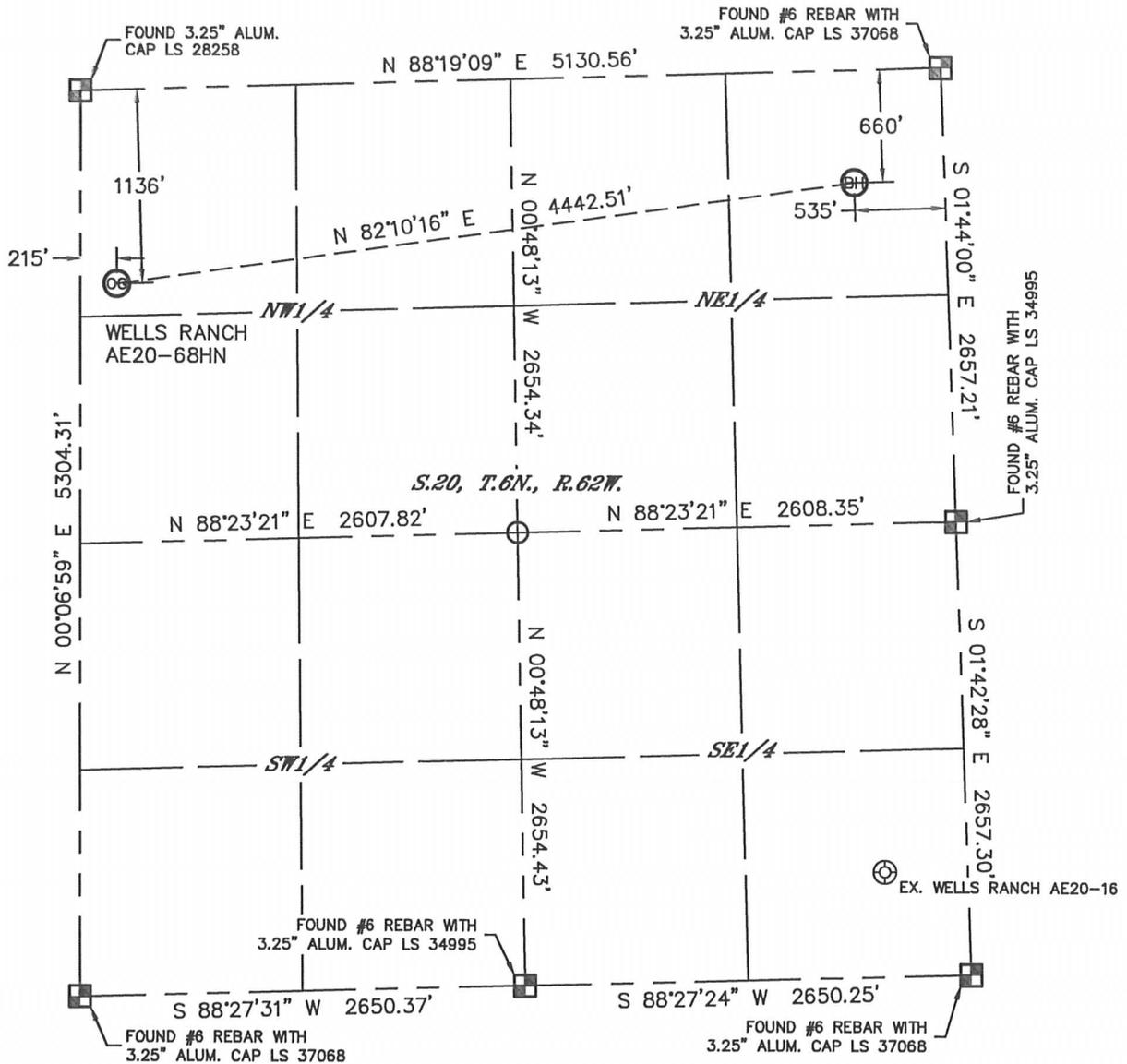
In accordance with a request from Brian James with Noble Energy Inc. Lat40°, Inc. has determined the surface location of the WELLS RANCH AE20-68HN to be 1136' from the NORTH line and 215' from the WEST line and the bottom hole to be 660' from the NORTH line and 535' from the EAST line as measured at right angles from the section lines of Section 20, Township 6 North, Range 62 West of the Sixth Principal Meridian, County of Weld, State of Colorado.
