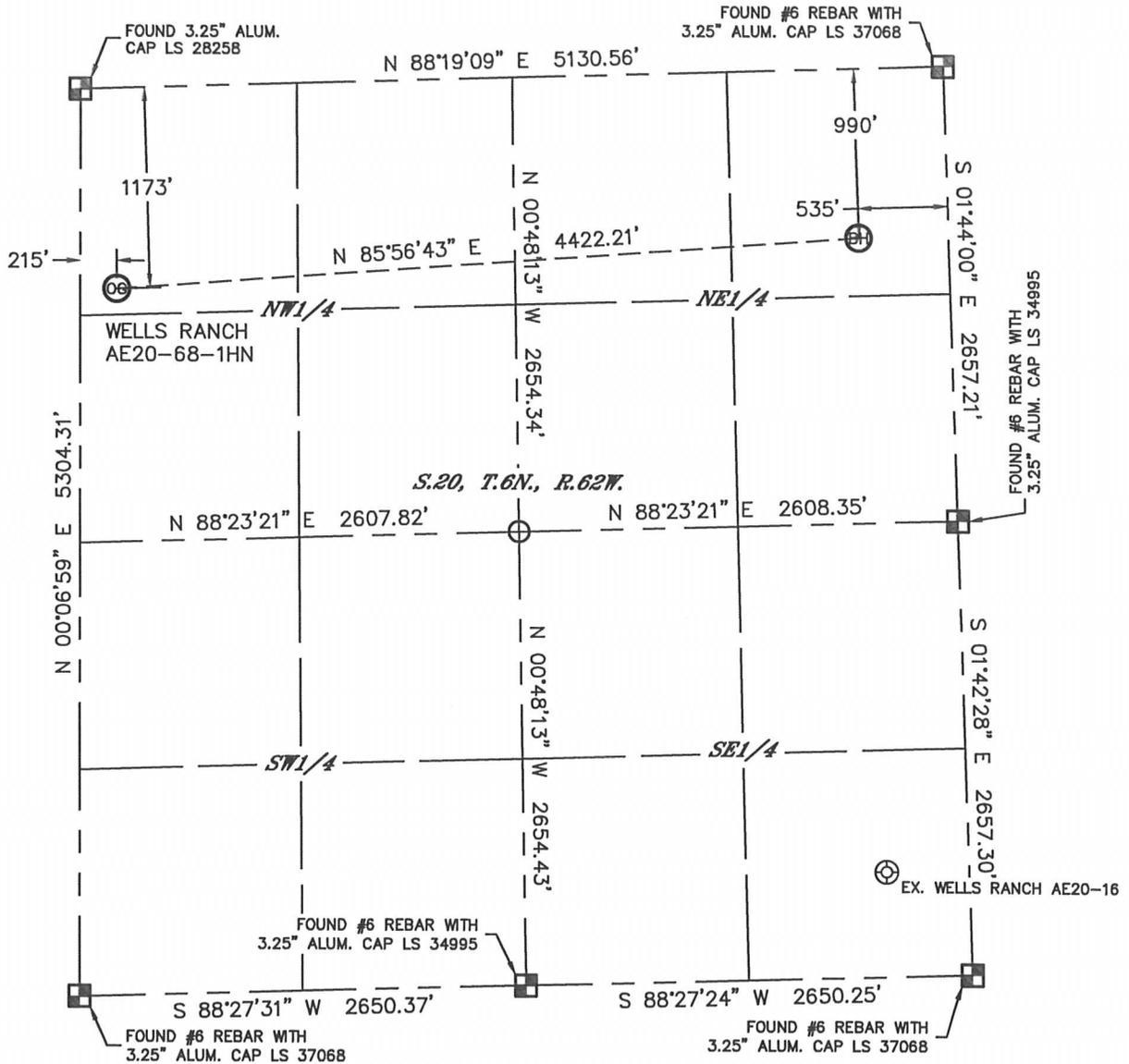
In accordance with a request from Brian James with Noble Energy Inc. Lat40°, Inc. has determined the surface location of the WELLS RANCH AE20-68-1HN to be 1173' from the NORTH line and 215' from the WEST line and the bottom hole to be 990' from the NORTH line and 535' from the EAST line as measured at right angles from the section lines of Section 20, Township 6 North, Range 62 West of the Sixth Principal Meridian, County of Weld, State of Colorado.
