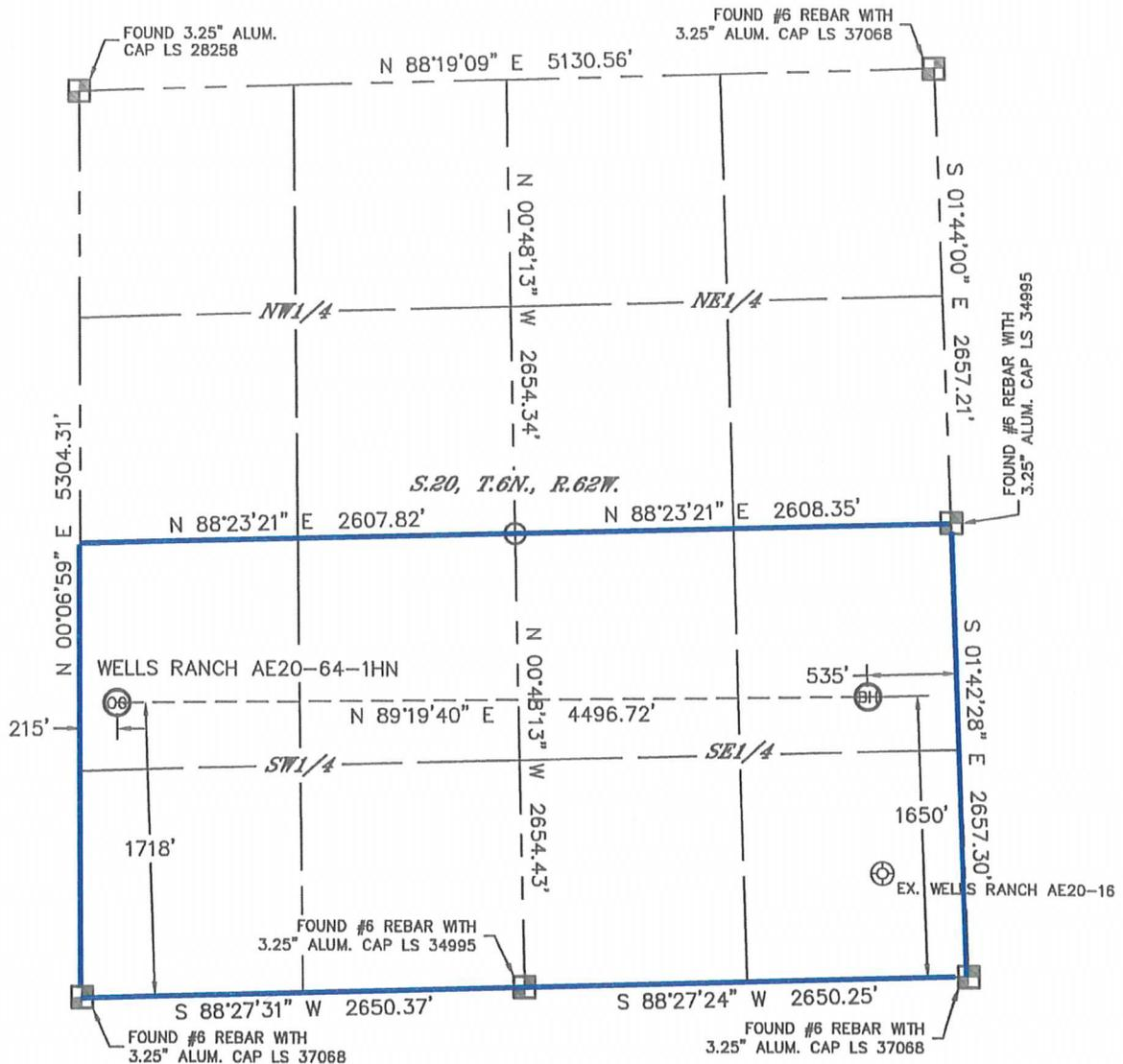
In accordance with a request from Brian James with Noble Energy Inc. Lat40°, Inc. has determined the surface location of the WELLS RANCH AE20-64-1HN to be 1718' from the SOUTH line and 215' from the WEST line and the bottom hole to be 1650' from the SOUTH line and 535' from the EAST line as measured at right angles from the section lines of Section 20, Township 6 North, Range 62 West of the Sixth Principal Meridian, County of Weld, State of Colorado.
