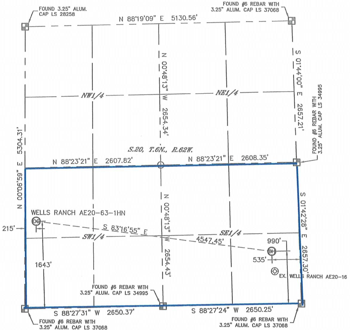
In accordance with a request from Brian James with Noble Energy Inc., Lat40°, Inc. has determined the surface location of the WELLS RANCH AE20-63-1HN to be 1643' from the SOUTH line and 215' from the WEST line and the bottom hole to be 990' from the SOUTH line and 535' from the EAST line as measured at right angles from the section lines of Section 20, Township 6 North, Range 62 West of the Sixth Principal Meridian, County of Weld, State of Colorado.
