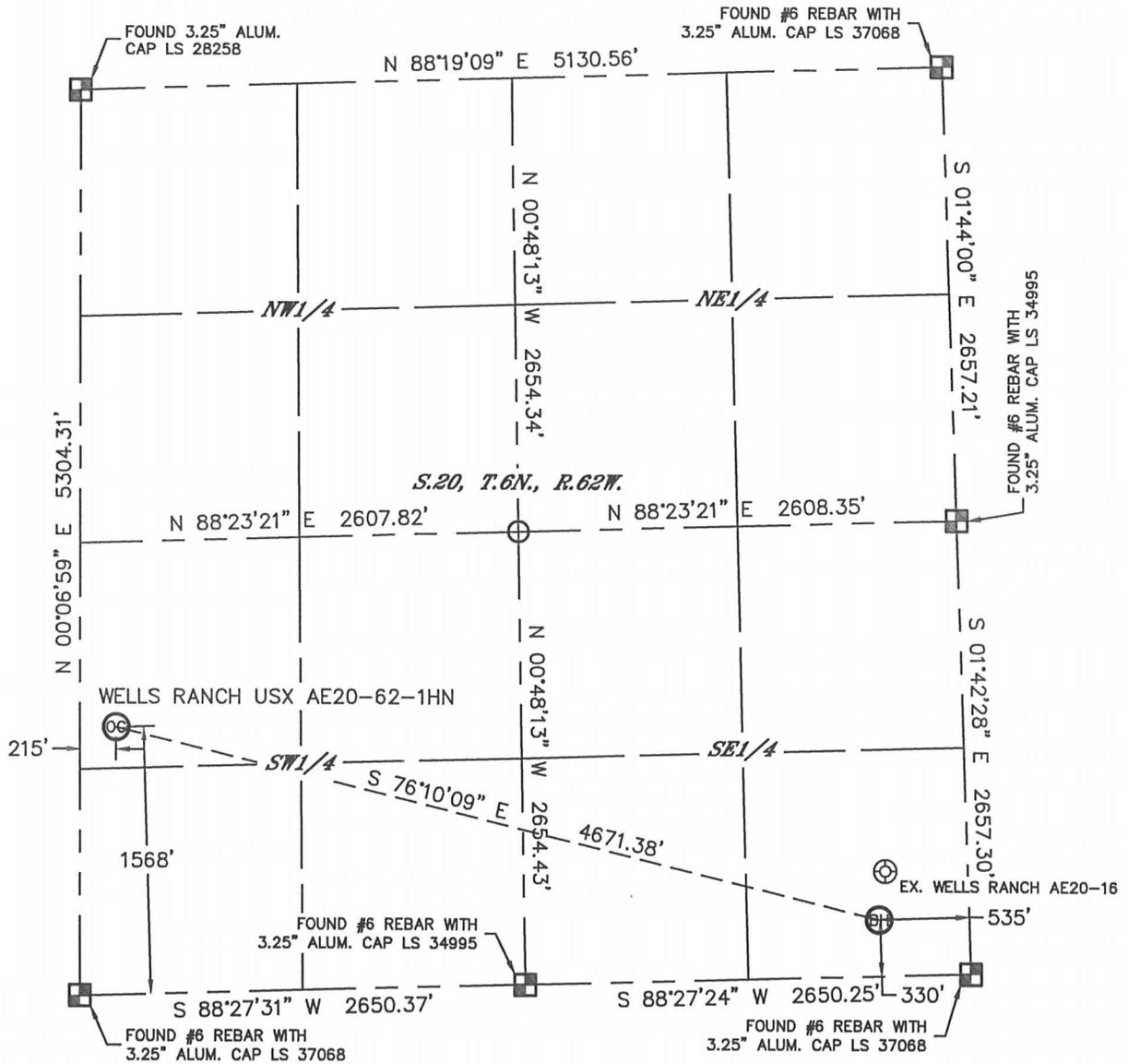
In accordance with a request from Brian James with Noble Energy Inc. Lat40°, Inc. has determined the surface location of the WELLS RANCH USX AE20-62-1HN to be 1568' from the SOUTH line and 215' from the WEST line and the bottom hole to be 330' from the SOUTH line and 535' from the EAST line as measured at right angles from the section lines of Section 20, Township 6 North, Range 62 West of the Sixth Principal Meridian, County of Weld, State of Colorado.
