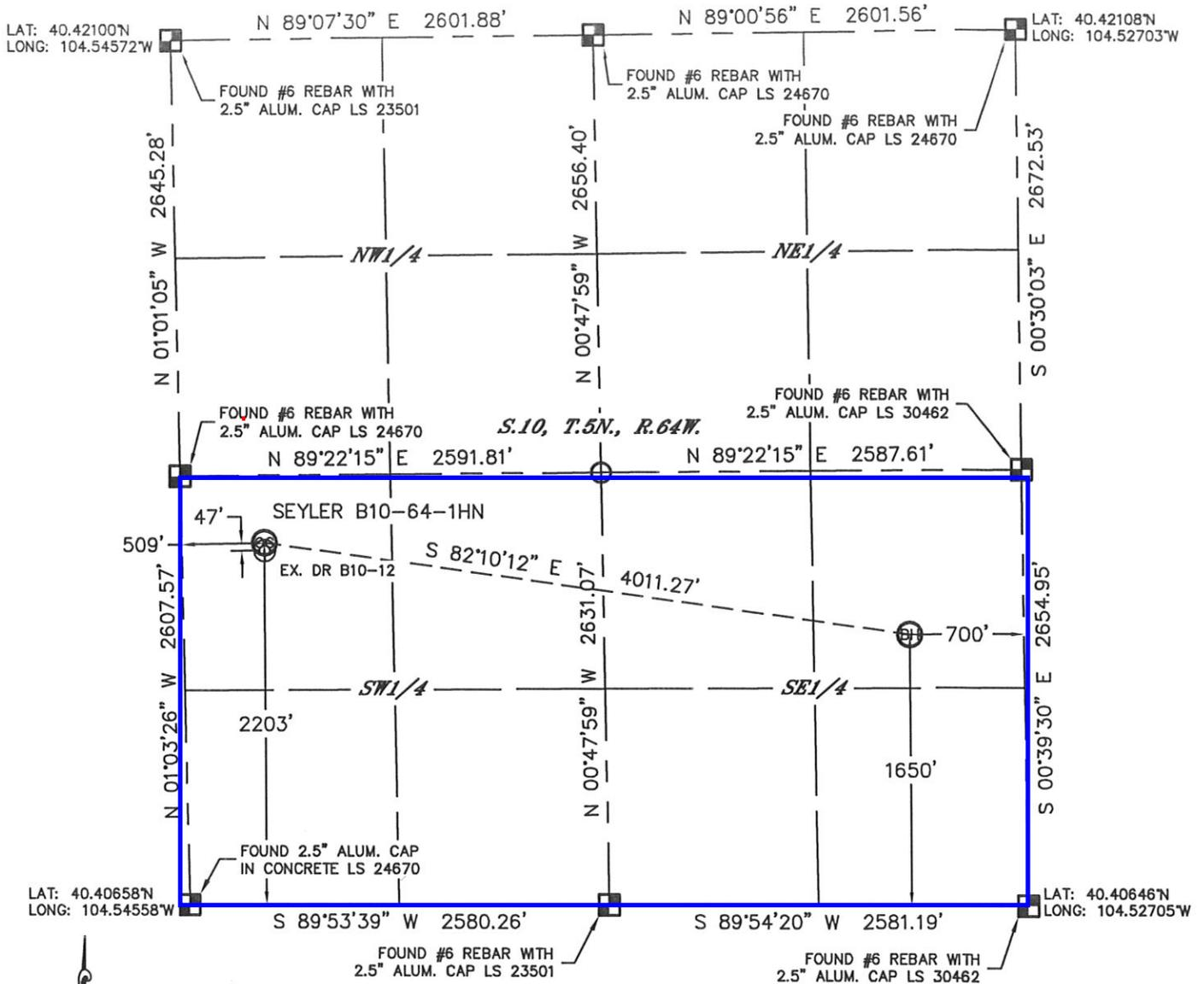
In accordance with a request from Jacob Rice with Noble Energy Inc. Lat40°, Inc. has determined the surface location of the SEYLER B10-64-1HN to be 2203' from the SOUTH line and 509' from the WEST line and the bottom hole to be 1650' from the SOUTH line and 700' from the EAST line as measured at right angles from the section lines of Section 10, Township 5 North, Range 64 West of the Sixth Principal Meridian, County of Weld, State of Colorado.
