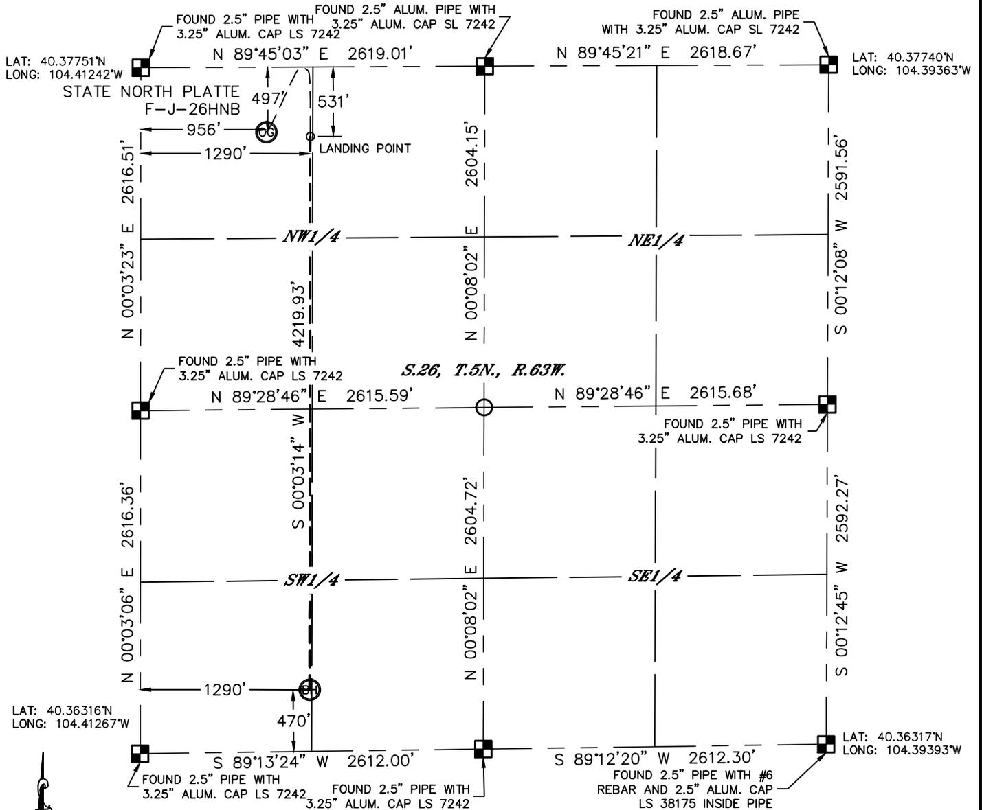
In accordance with a request from Michael Meagher with BONANZA CREEK ENERGY, INC. Lat40°, Inc. has determined the surface location of the STATE NORTH PLATTE F-J-26HNB to be 497' from the NORTH line and 956' from the WEST line and the bottom hole to be 470' from the SOUTH line and 1290' from the WEST line as measured at right angles from the section lines of Section 26, Township 5 North, Range 63 West of the Sixth Principal Meridian, County of Weld, State of Colorado.
