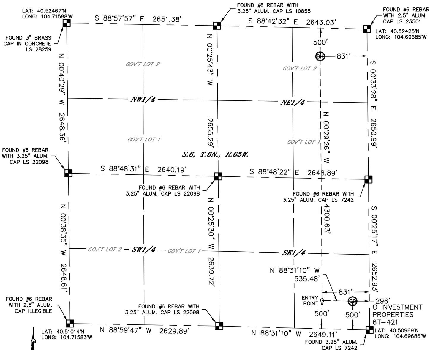
In accordance with a request from Jeff Dillingham with PDC ENERGY Lat40°, Inc. has determined the surface location of the O INVESTMENT PROPERTIES 6T-421 to be 500' from the SOUTH line and 296' from the EAST line and the bottom hole to be 500' from the NORTH line and 831' from the EAST line as measured at right angles from the section lines of Section 6, Township 6 North, Range 65 West of the Sixth Principal Meridian, County of Weld, State of Colorado.
