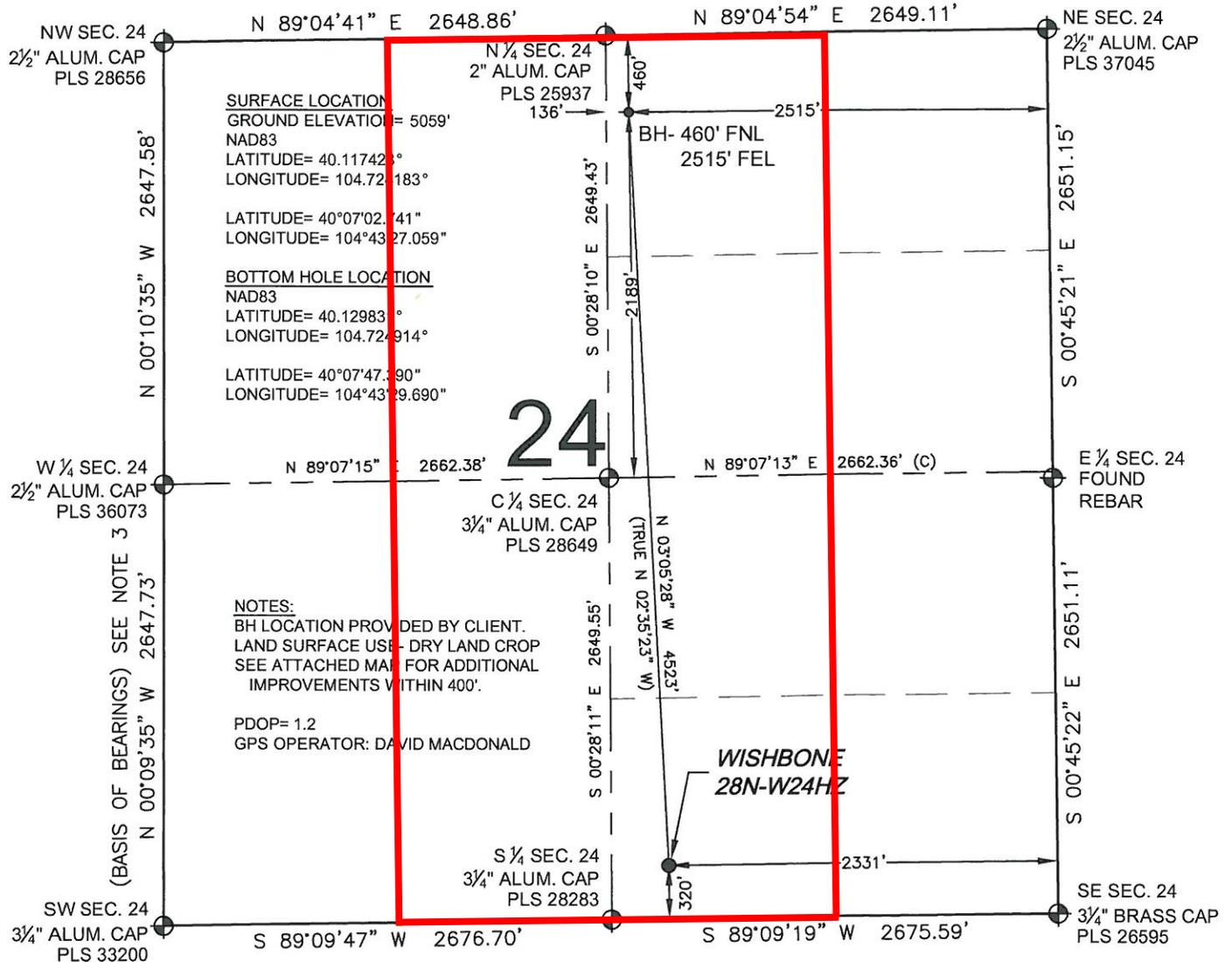
WELL WISHBONE 28N-W24HZ TO BE LOCATED 320' FSL AND 2331' FEL
