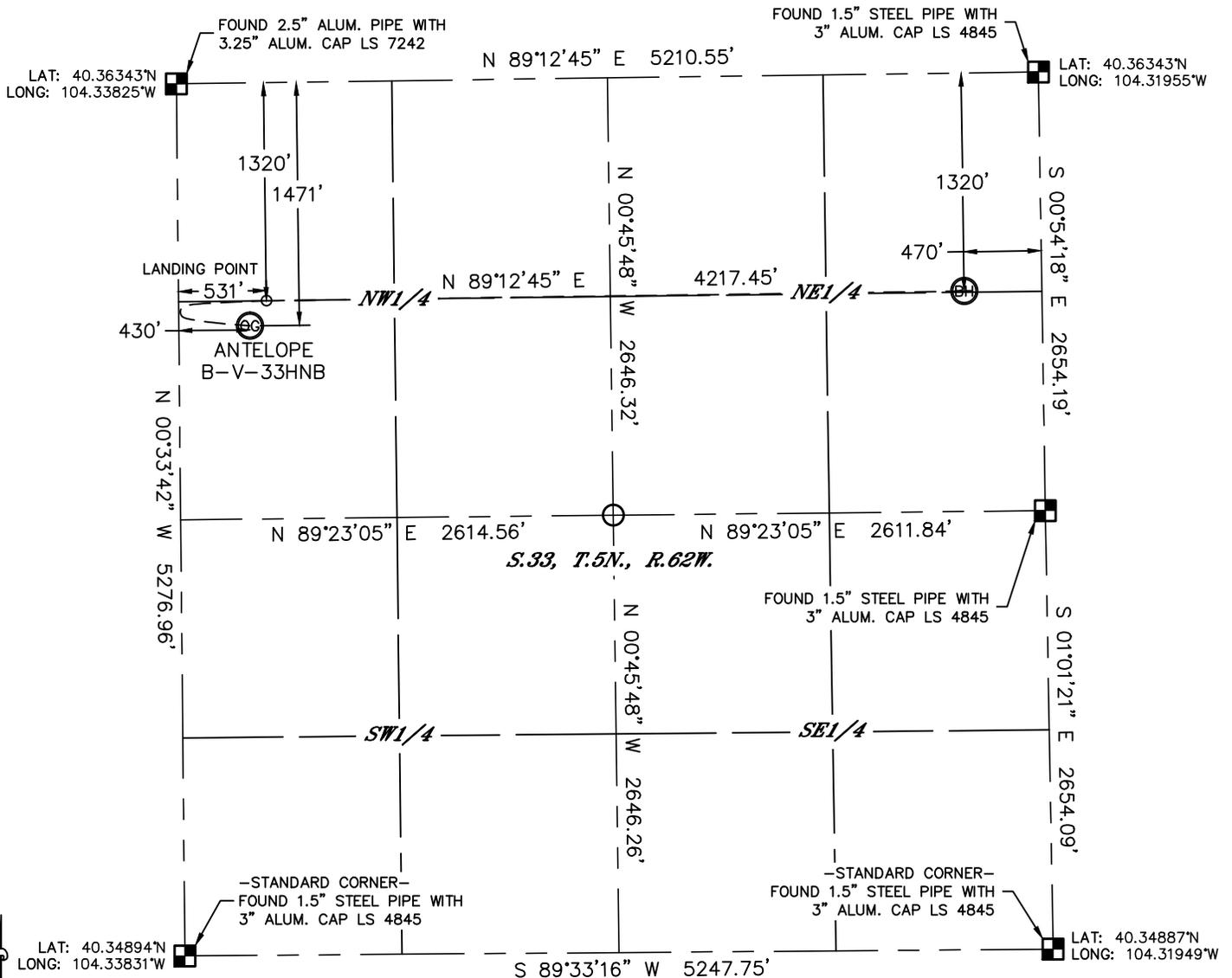
In accordance with a request from Michael Meagher with BONANZA CREEK ENERGY, INC. Lat40°, Inc. has determined the surface location of the ANTELOPE B-V-33HNB to be 1471' from the NORTH line and 430' from the WEST line and the bottom hole to be 1320' from the NORTH line and 470' from the EAST line as measured at right angles from the section lines of Section 33, Township 5 North, Range 62 West of the Sixth Principal Meridian, County of Weld, State of Colorado.
