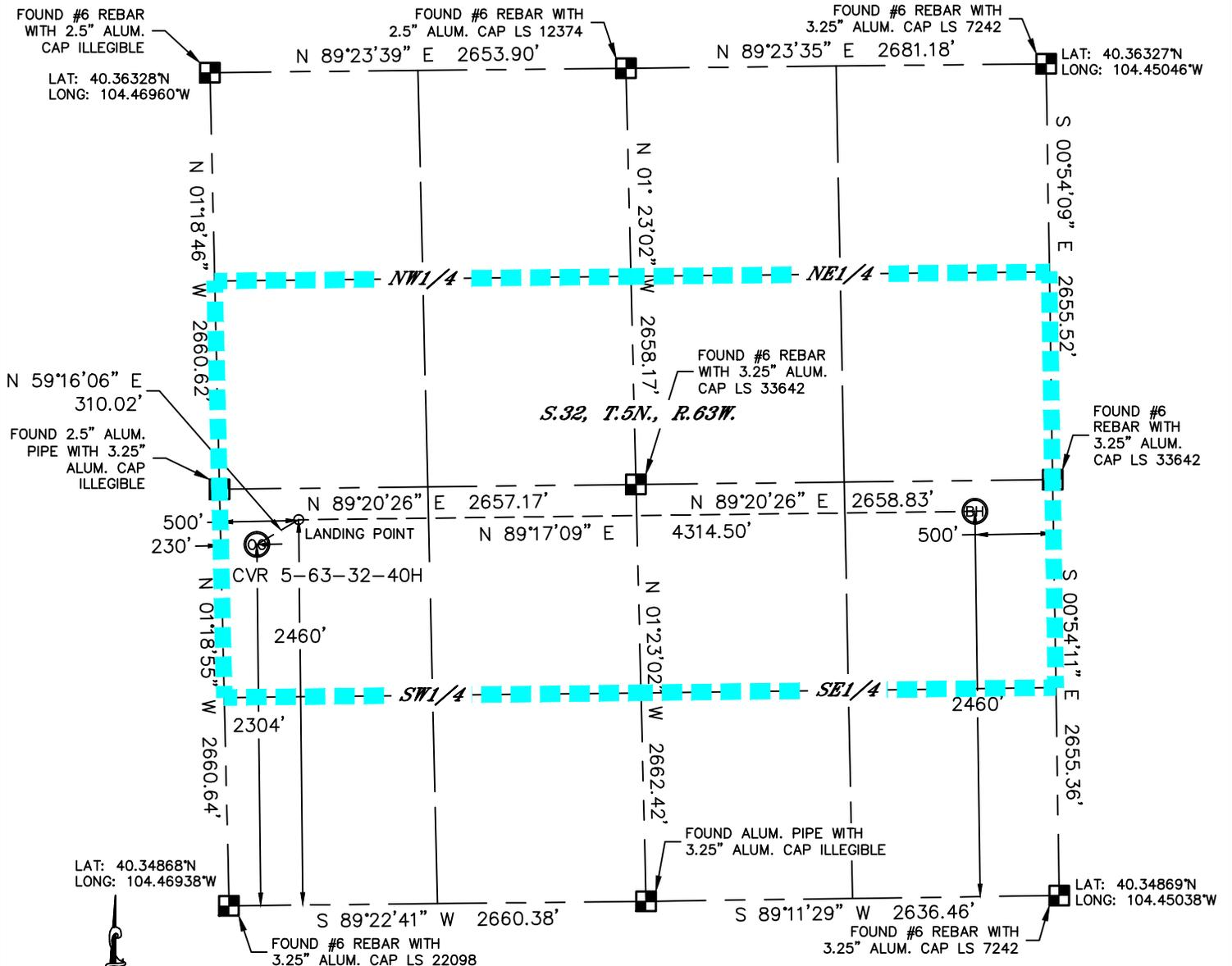
In accordance with a request from Glenn Berglund with BILL BARRETT CORPORATION Lat40°, Inc. has determined the surface location of the CVR 5-63-32-40H to be 2304' from the SOUTH line and 230' from the WEST line and the bottom hole to be 2460' from the SOUTH line and 500' from the EAST line as measured at right angles from the section lines of Section 32, Township 5 North, Range 63 West of the Sixth Principal Meridian, County of Weld, State of Colorado.
