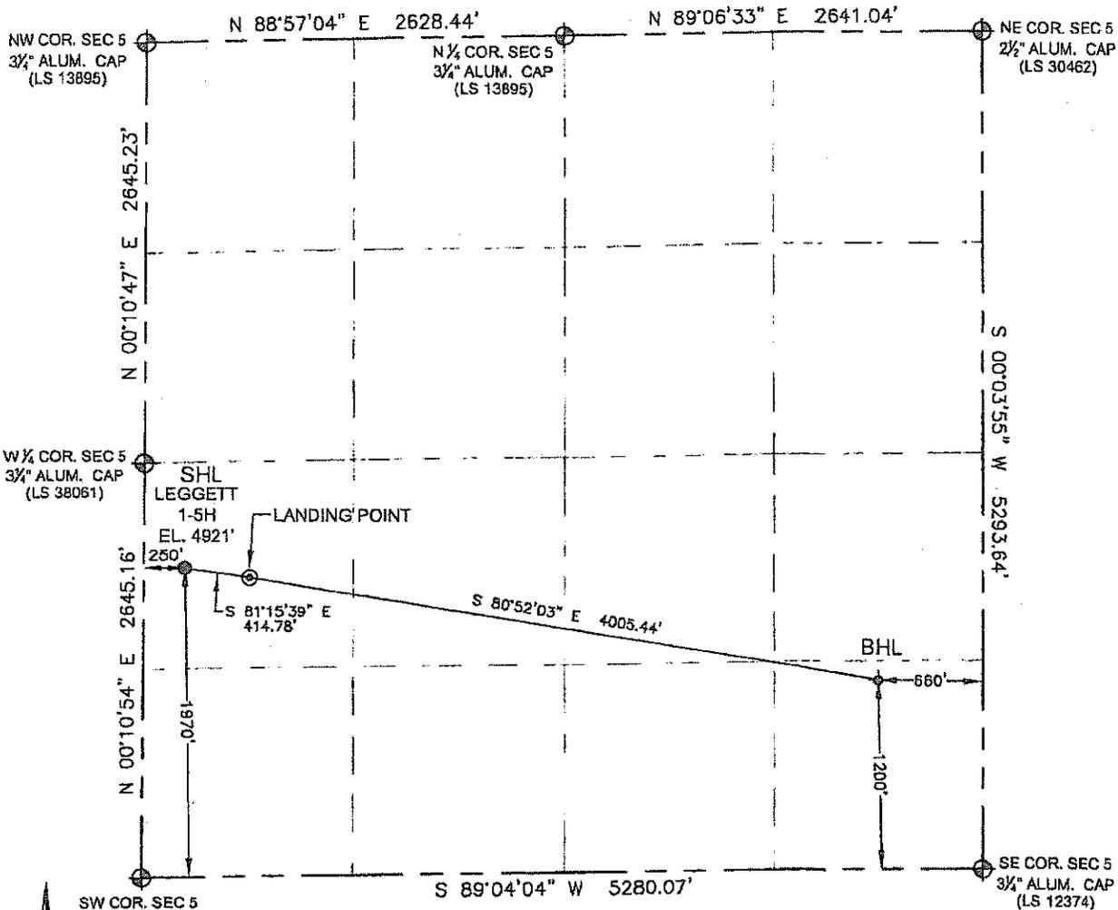
In accordance with a request from Lance Harper with Continental Resources, Petroleum Field Services, LLC has determined the surface location of the LEGGETT 1-5H to be 1970' from the SOUTH line and 250' from the WEST line and the bottom hole to be 1200' from the SOUTH line and 660' from the EAST line as measured at right angles from the section line of Section 5, Township 7 North, Range 60 West of the Sixth Principal Meridian, County of Weld, State of Colorado.
