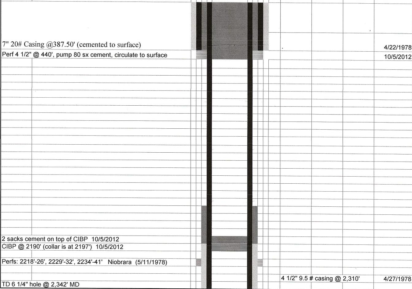
7" 20# Casing @387.50' (cemented to surface) 4/22/1978
